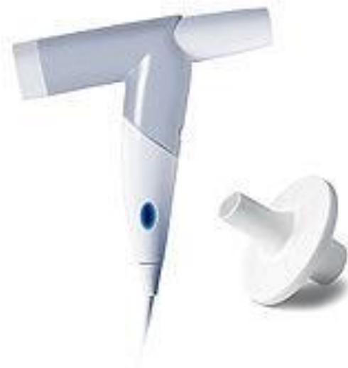
A modern USB PC-based spirometer
